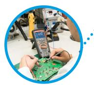
The meter allows the measurement of very small currents in the range of  $500 \,\mu$ A, useful during service works, e.g. in tests of real-time clock support systems or in the maintenance of flame sensors in combustion chambers.
