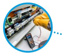
Measurements of the current loop 4-20 mA in analogue circuits controlling temperature, pressure, humidity or flow sensors are possible thanks to the special function that displays the percentage results for the corresponding current values.
